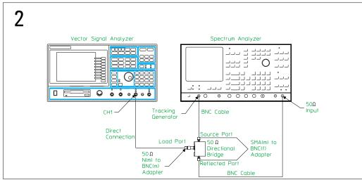
Verifying Specifications To set up the input rtn loss test
