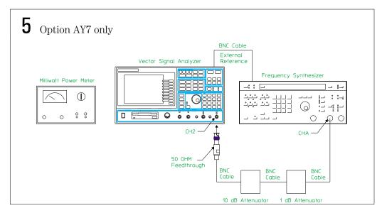
Verifying Specifications To set up the amplitude accuracy test
