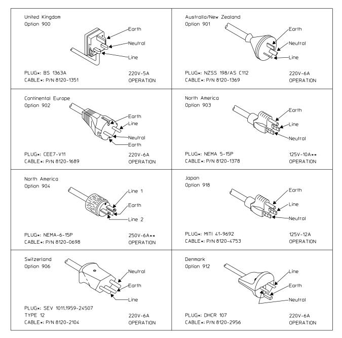
\*The number shown for the plug is the industry identifier for the plug only, the number shown for the cable is an Agilent part number for a complete cable including the plug.
