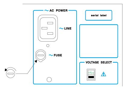
**3** Pull the fuse from the fuse holder cap.
